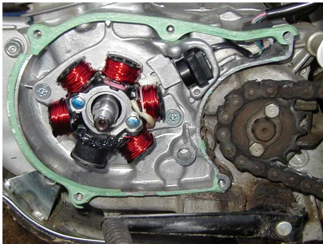
The stator with the new windings installed back into the bike.
