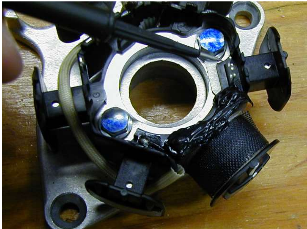
Here is a test probe pointing at the ground terminal
