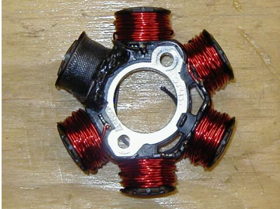
The stator, with the new windings
